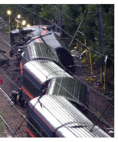
to damage than others. When an increase in the manufacturing hardness of rails is added to changes to the wheel profile that meant the same section of rail was being used all the time, an accident was much more likely.
