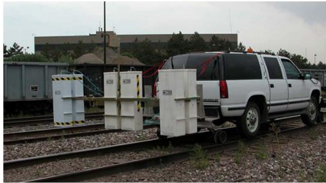
FIGURE4. 9 – GPR RAIL-SETUP WITH THREE PAIRS OF 1-GHZ HORN ANTENNAS (SELIG ET AL., 2003).
