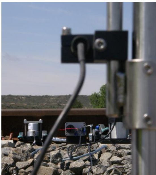
FIGURE 4.7 – LASER SYSTEM USED FOR MEASURING RAIL DEFLECTIONS DIRECTLY
