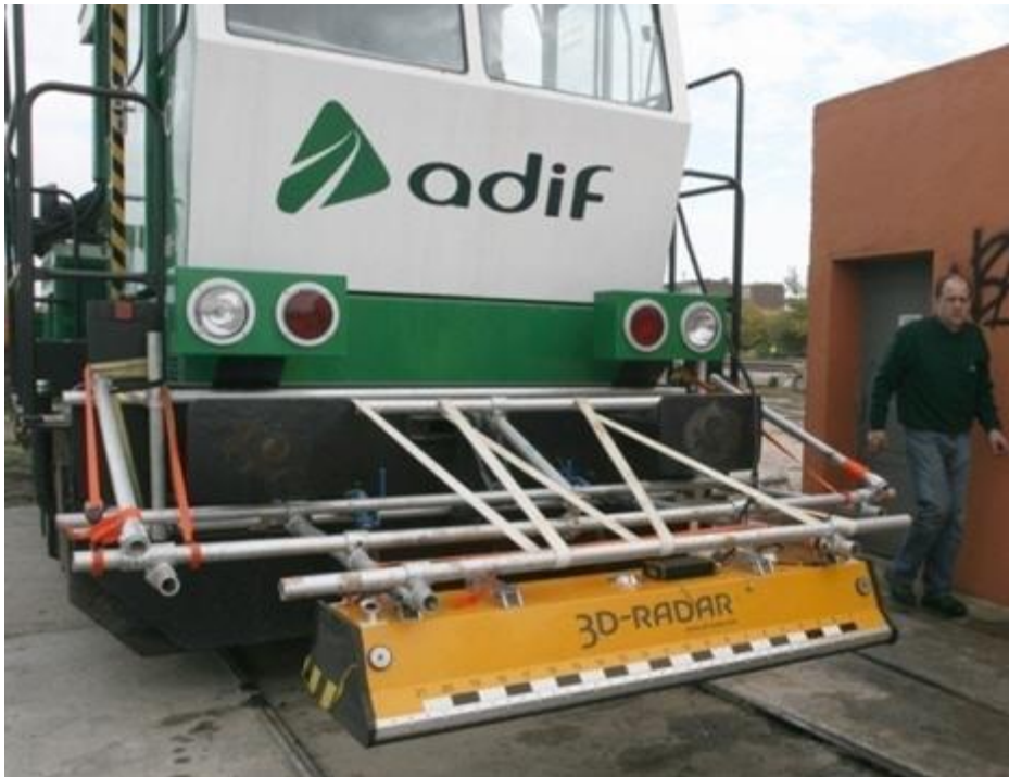
FIGURE 4.12. 3D-RADAR GPR SYSTEM TESTED MOUNTED ON THE FRONT OF AN ADIF MAINTENANCE TRAIN.
