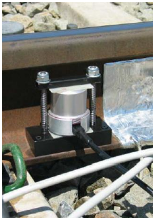
FIGURE 4.8 – GEOPHONE OF 2 HZ PROVIDED WITH THE ADEQUATE SUPPORT TO BE CLAMPED TO THE BASE OF A STANDARD RAIL
