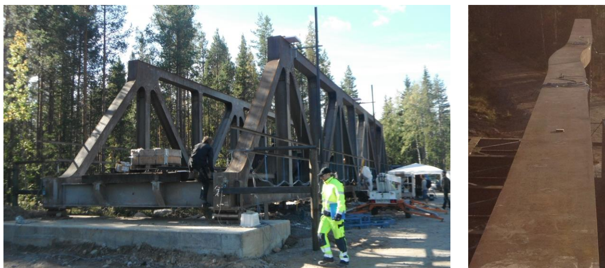
FIGURE 5.18 TEST OF 55 YEAR OLD 33 M LONG METALLIC BRIDGE AT ÅBY RIVER IN 2013. OVERVIEW OF TEST SITE WITH TWO JACKS ANCHORED IN THE BED ROCK IN THE CENTRE (LEFT) AND FINAL BUCKLING FAILURE OF TOP GIRDER BEAM (RIGHT), ML-D1.3 (2015), HÄGGSTRÖM ET AL (2016, 2017).
