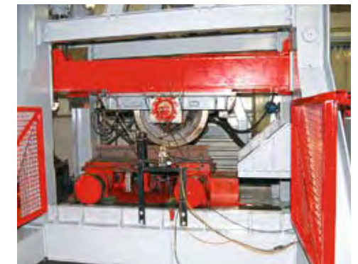
Figure 5.4.1-1: Left: twin disk test rig (SUROS), right: linear test rig (VAS)
