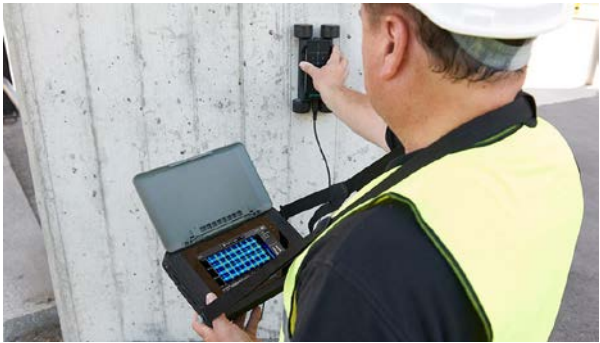
Figure B.9 Use of cover meter, from ( http:// www.proceq.com )
